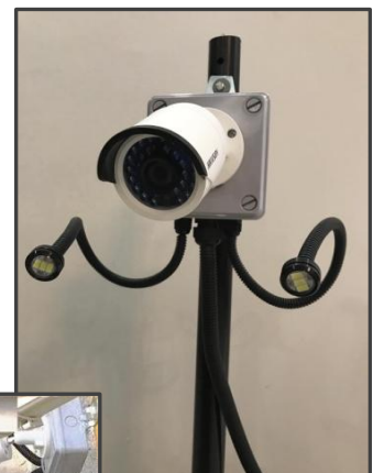
CCTV complete with 2 No. LED lights
